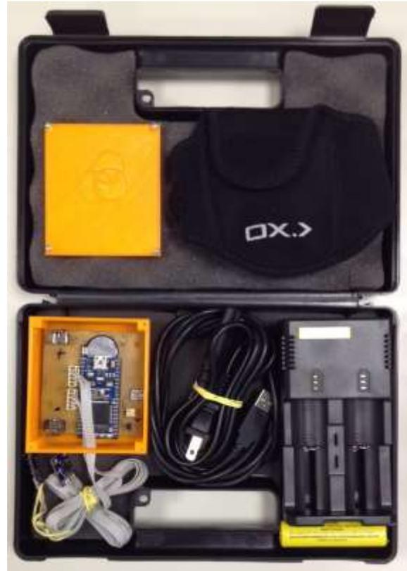
**Figure 3:** PG box showing its components; PG open enclosure on the left; cables at the center; battery and charger on the right side.
